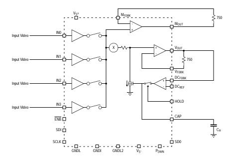
500MHz Video Front End: 4-1 MUX, VGA & DC-Restore
